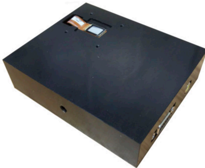
Figure 4.5: Cambridge Correlators TN-LC SLM SDE1024.
