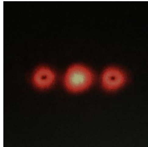
Figure 3.11: Long distance propagation photo for |l| = 2 fork CGH with G = 15 (4 px per fringe which is about 40 m in our SLM) using the setup shown in figure 4.6 without a polariser.
